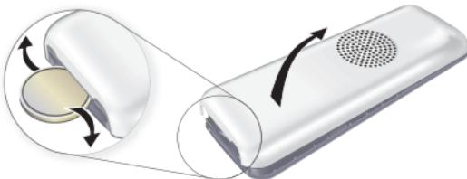
2. Insert the battery. The conductors of the battery must be in contact with the conductors in the housing.
